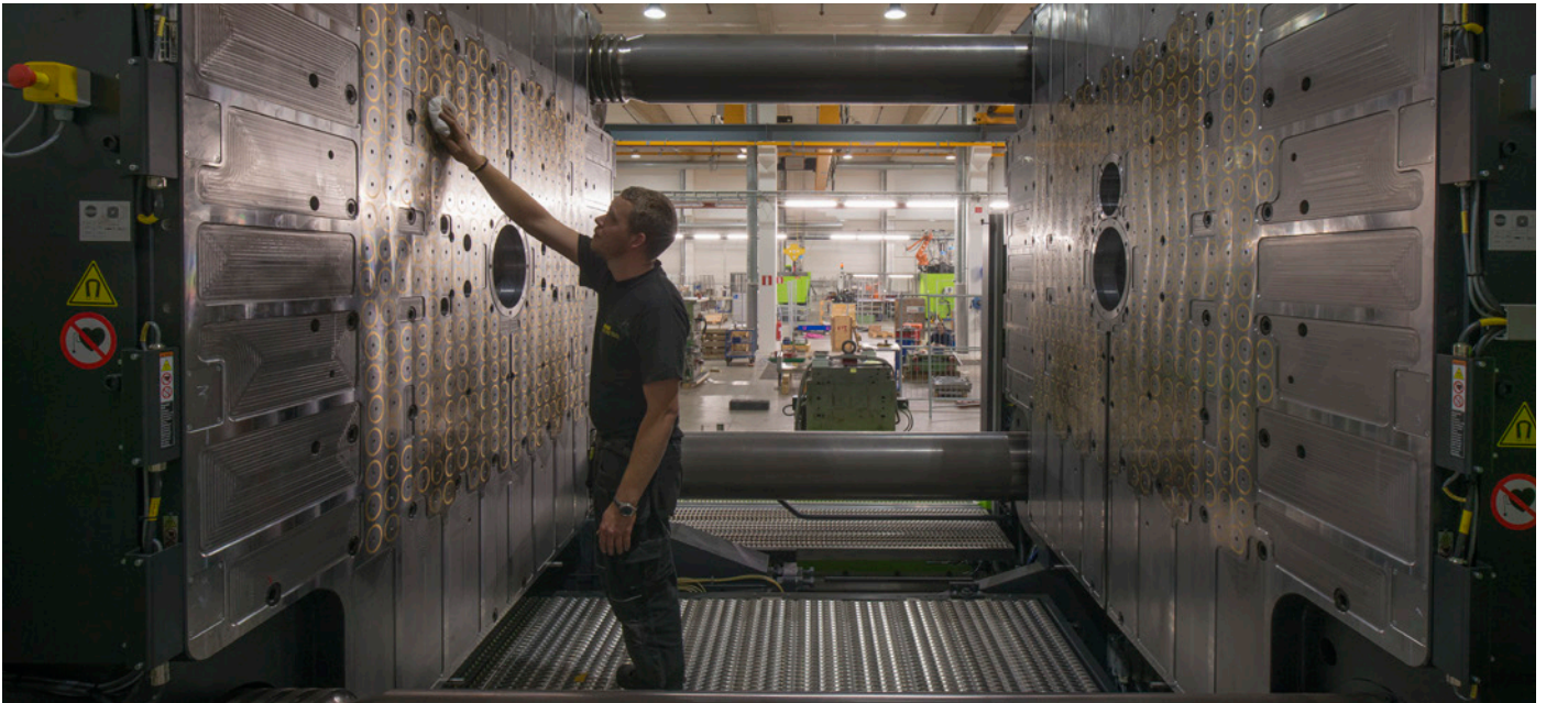
The size of the machine can be seen as a production fitter prepares the new mould. He is standing where the mould will hang.
