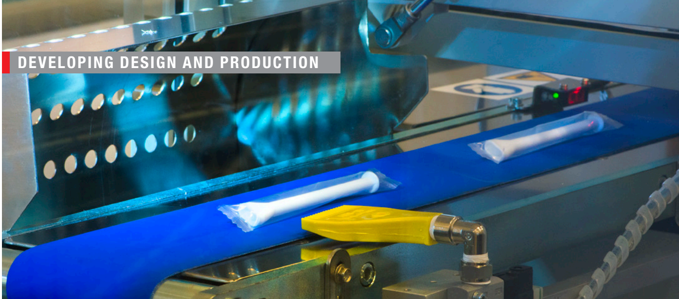
The applicator is manufactured using a fully automated, continual process that also includes individual and batch packaging.
