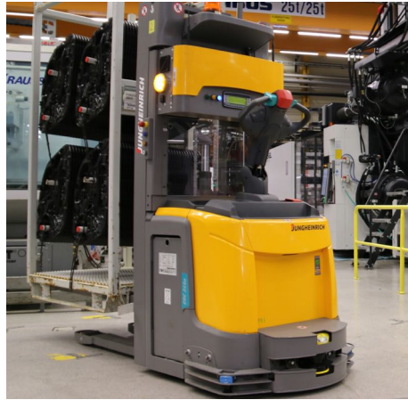
Efficiency is gained from driverless forklifts and mould maintenance right next to the injection mould machines.
