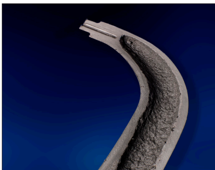
The gas pushes the plastic against the sides of the mould, creating a cavity.
