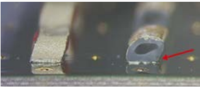
Figure 5. Nolato (left) and reference (right) pads after compression to 31 % and damp heat steady state (1000 h, 85 °C / 85% RH) ageing. The arrow is indicating a crease in the surface foil of the reference pad.
