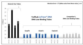
High Ct in real time PCR indicates high loss of DNA during sample preparation with normal grade tubes.
